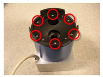
3. Remove the housing adapter from the IPA module.
