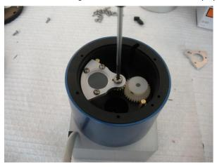
5. Remove the Polystyrene holder assembly.
