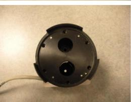
4. Secure with (6) 2-28 x  $\frac{1}{4}$ " TORX screws to a snug fit. Be careful not to over tighten as this could cause damage to the housing assembly.
