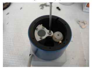
3. Reinstall housing adapter. Notice that the housing adapter is pinned. Carefully attach the housing adapter in the proper orientation.
